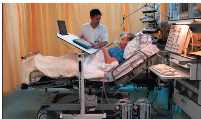
Photo 3. The 'communication car' is mobile. The height and surface angle are both adjustable so that the patient can operate the aid when lying in bed as well as sitting in a chair
